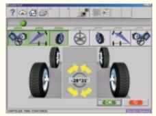
If operator still continues to turn the wheel, the machine knows that a full turn measurement (lock to lock) is wanted and continues on accordingly.
