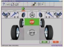
If the operator stops turning the wheel after the basic caster swing, the machine concludes that this is all the operator wants to do and proceeds on to the measurement screen
