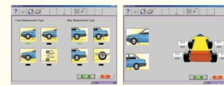
After selecting the manufacturer's recommended method for measuring ride height, actual ride heights can be measured and entered into the software for the specific vehicle being aligned. The vehicle's alignment specifications are then automatically modified to reflect the specific ride heights for the vehicle being aligned.
