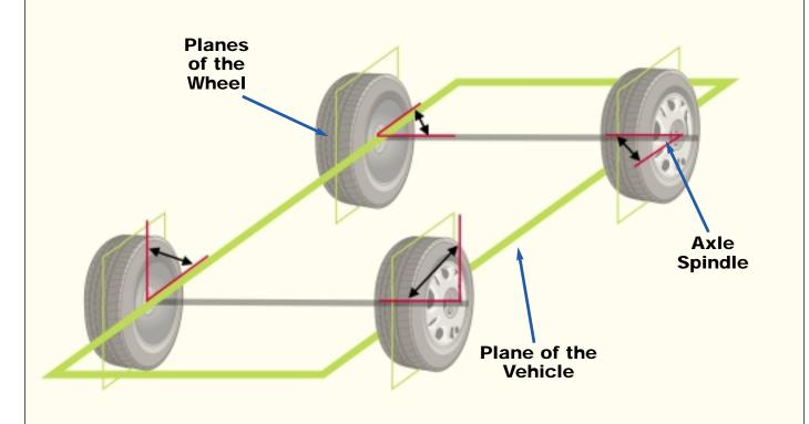
Using high resolution digital cameras and patented three dimensional modeling technology, the vertical planes of each of the vehicle's wheels as well as the plane of the vehicle itself are modeled. The vehicle's plane is modeled from the center points of each spindle axis where the wheels attach to the vehicle.
