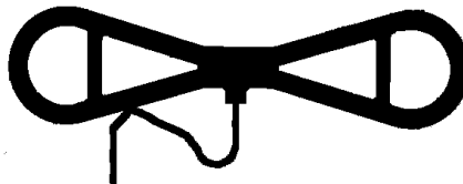
Figure 4, Antenna Tie Wrap Modification
