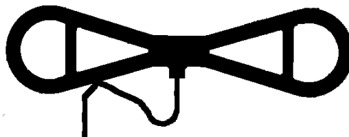
Figure 1, Antenna Tie Wrap Modification
