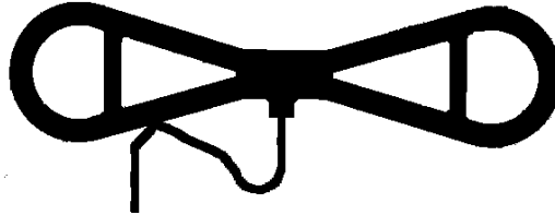
Figure 2, Antenna Tie Wrap Modification
