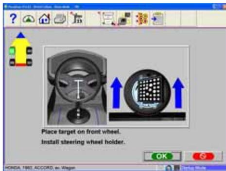
**Step 4.** Place the Target on the Corresponding Wheel
