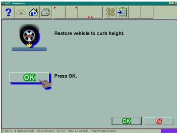
Figure 84. Lower Vehicle After Elevated SAI
