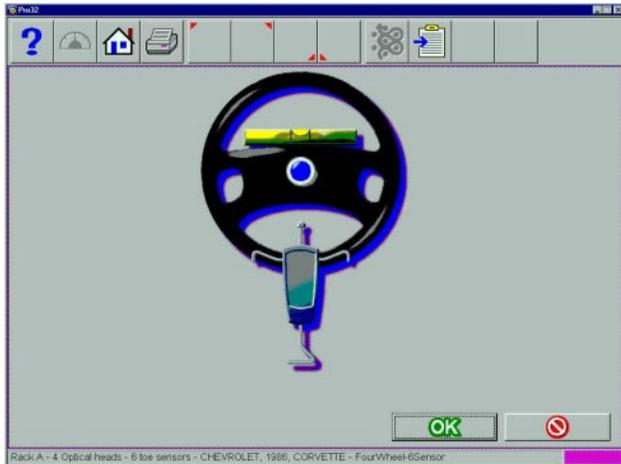
**Figure 66. Level and Lock Steering Wheel**
