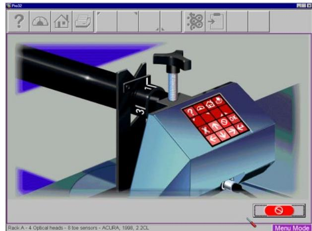
**Figure 128. Position 1, 2, 3 at 12:00 for Runout**
