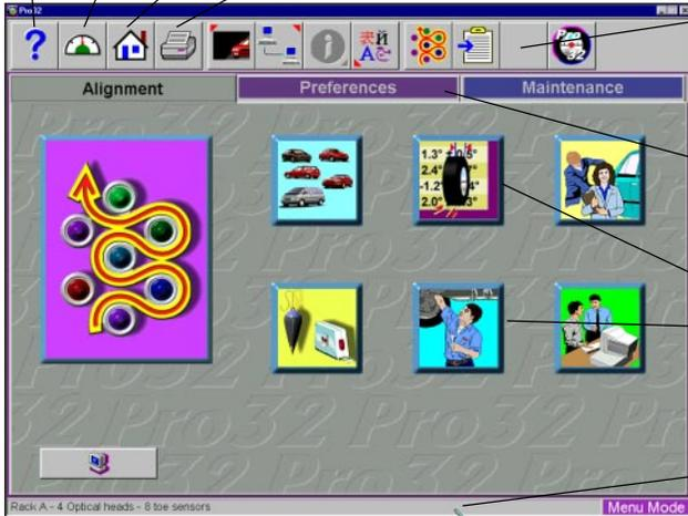
**Toolbar** – these buttons appear on every screen, and correspond to the F1-F12 keys on the keyboard, as well as the keys on the remote. The functions for F1-F4 are common to every screen, while the functions of F5-F12 vary depending on the screen
