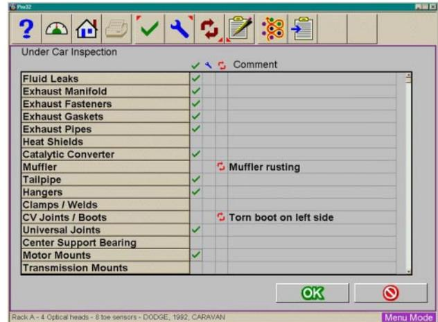
Figure 50. Undercar Inspection
