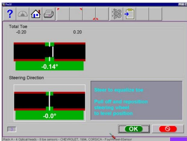
Figure 114. Single Tie Rod Adjust Screen
