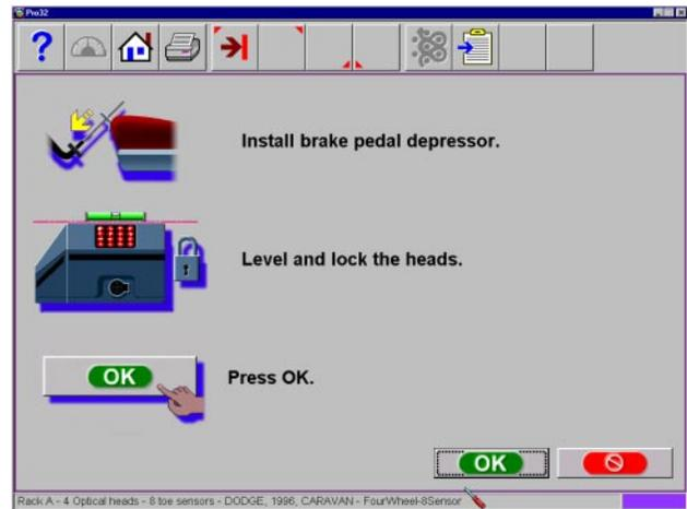
**Figure 81. Lock Brakes and Heads**
