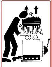
An exploding tire and rim may be propelled upward and outward with enough force to cause serious injury or death. This tire changer is not a safety device and will not restrain exploding tires and rims.
