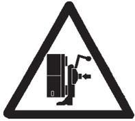
Risk of crushing. Stand clear of bead breaker arm during operation.
