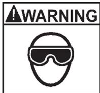
Risk of eye injury. Flying debris, dirt, and fluids may be discharged during bead seating and inflation process.
