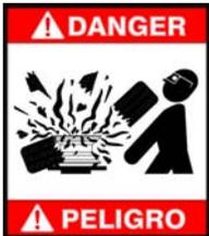
Overinflated tires or tires mounted on the wrong sized rims can explode producing hazardous flying debris.
