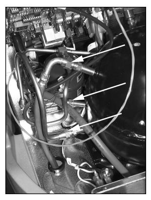
Figure 3-3: Pump Connections
