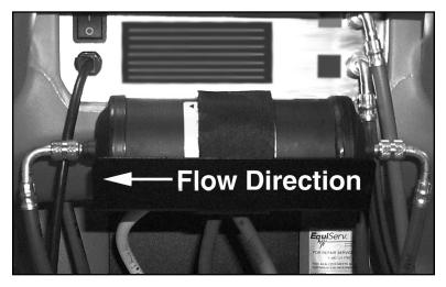
Figure 3-1: Master Filter/Dryer
