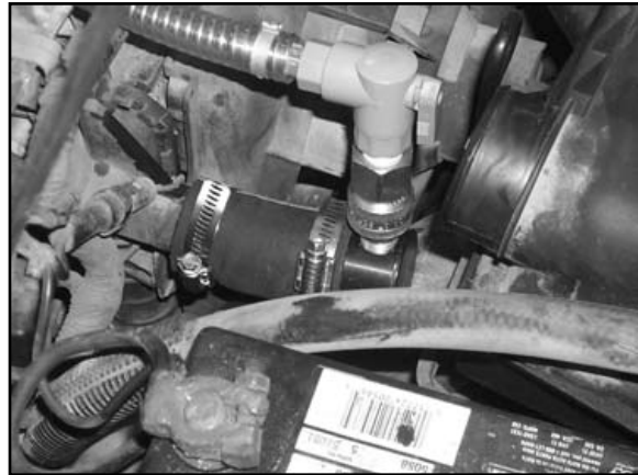
Figure 5: Recovery Hose and Adapter Attached to Radiator
