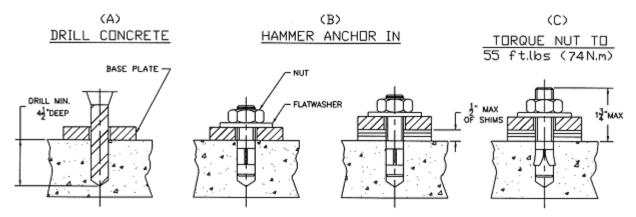
Figure 9 - Anchoring
