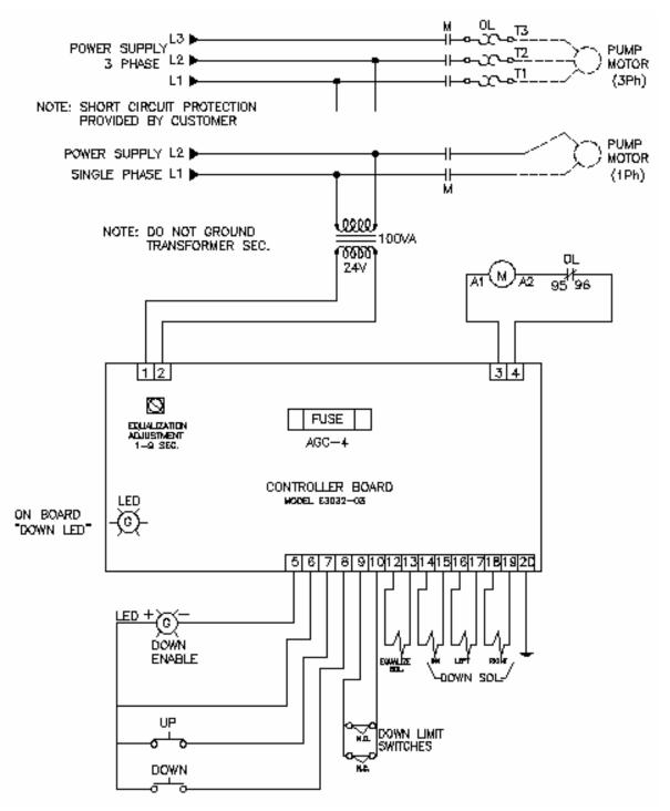
Figure 5 - Electrical Schematic
