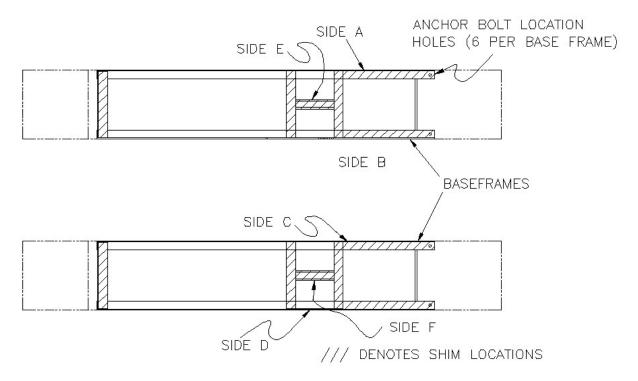
Figure 8 - Leveling Procedure Example
