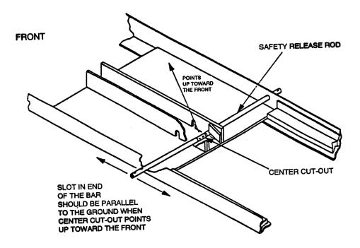
Figure 7 - Safety release rod location.
