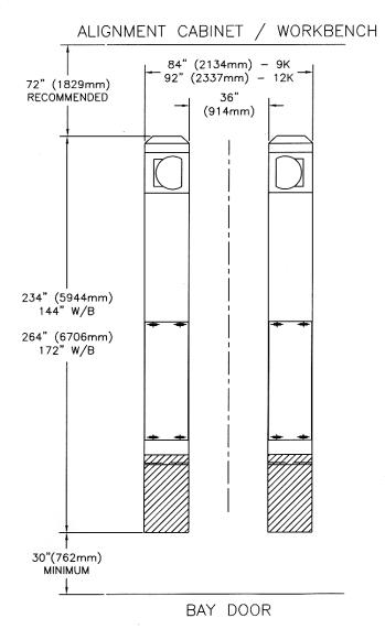
Figure 2 - Typical bay layout (surface mount)
