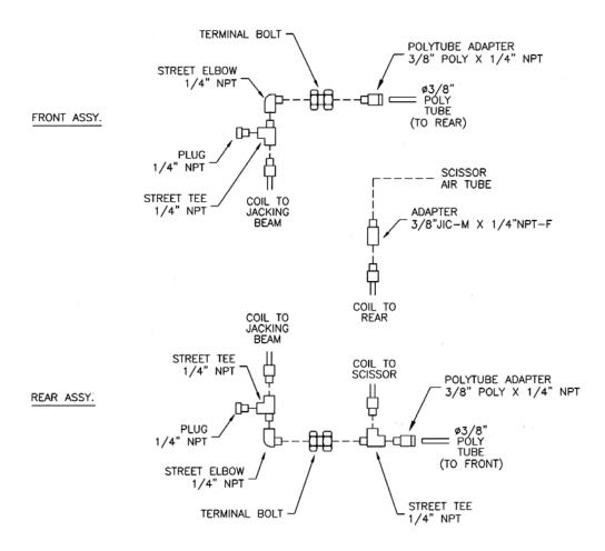
**Figure 6 – Air Line Connections**
