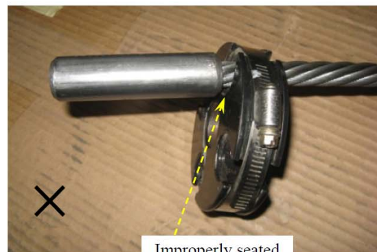
Improperly seated Cable exposed
