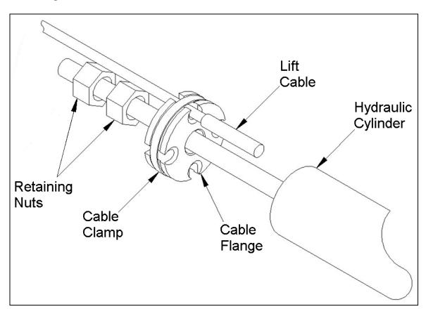
Figure 8. Cable Installation at Flange
