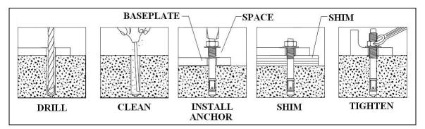
Figure 11. Anchor installation
