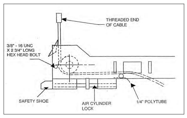
Figure 3. Typical cable routing in crossmember assembly
