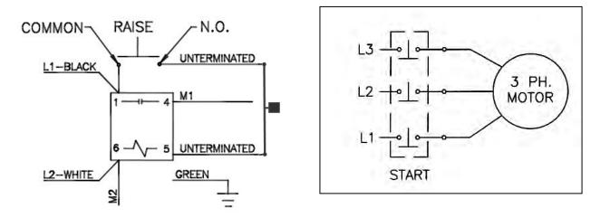
Figure 7. Electrical diagram for 230V/1 Ph and 230V/3 Ph
