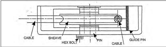
Figure 5. Sheave stack
