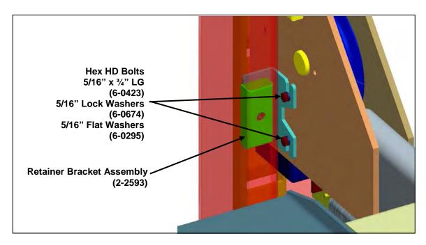
Figure 9. Retainer bracket installation
