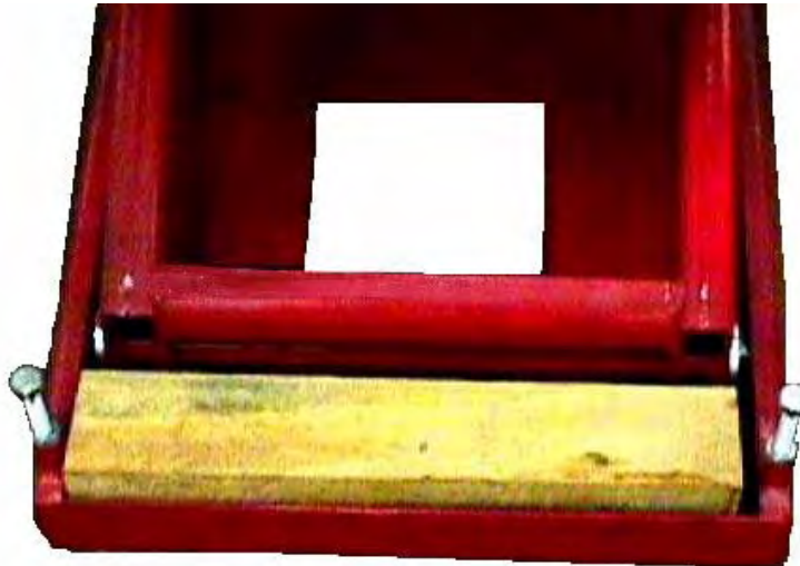
Figure 3 – Insert 4”x4” Wood Block as a Safety Mechanism During Installation
