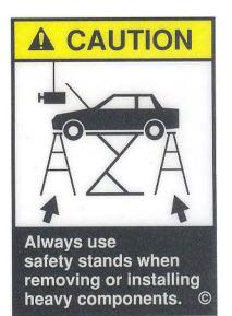
**DANGER:** If the lift should become stuck at any raised position, do not attempt to lower the lift by loosening any hydraulic fittings. Contact technical services at 1-800-268-7959.
