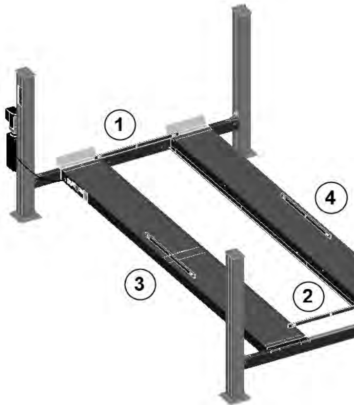
Figure 20 - Lift & Deck Leveling
