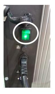
When the power switch is turned on, the unit initiates the system boot-up. This boot sequence will take a few moments.
