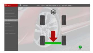
Once the vehicle has returned to the start position, compensation is complete. If changes were detected in one or more suspension angles the screen will alert the user to roll the vehicle to relieve stress and then to perform
