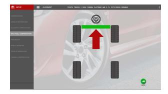
Move the vehicle forward as indicated. The arrow will again turn red when the correct position is reached.
