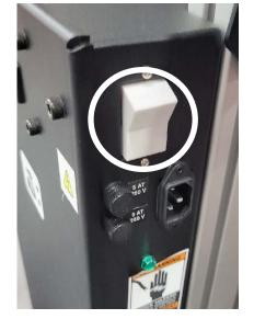
When the power switch is turned ON, the unit initiates the system boot-up. This boot sequence will take a few moments.
