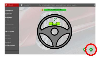
forth to achieve level. *Note:* Be sure the turntable lock pins have been removed prior to leveling. Click on "Done" to advance to Caster measurement.
