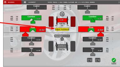
Specifications for the vehicle under test are shown on the screen with minimum, maximum and preferred values. The actual live value is shown inside the measurement block. Cross values, total toe and thrust angle are displayed in the center of the screen.
