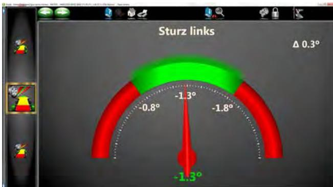
The left rear camber comparator in detail.
