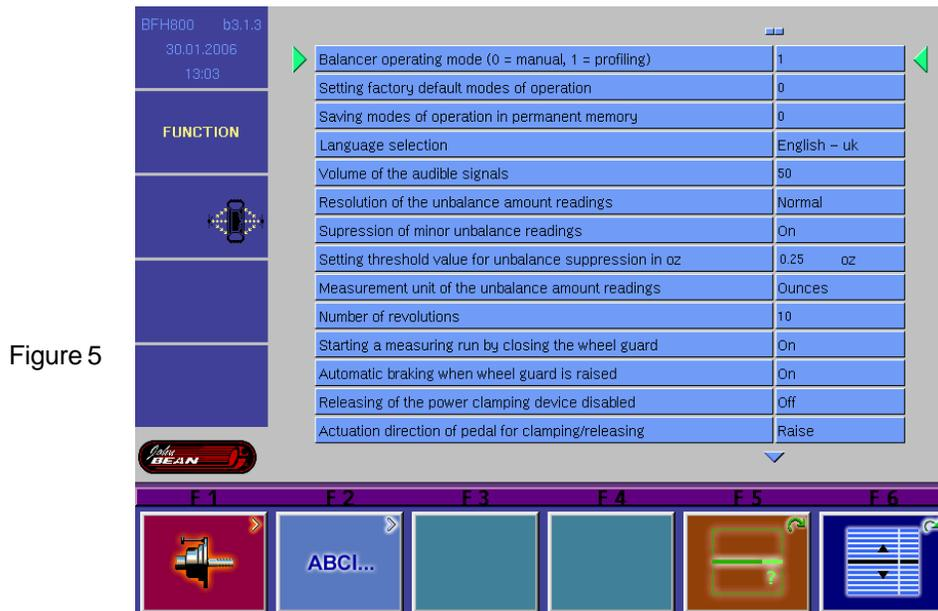
**B.** Press and hold the “F6” button and rotate the wheel to scroll up or down to the desired line item.
