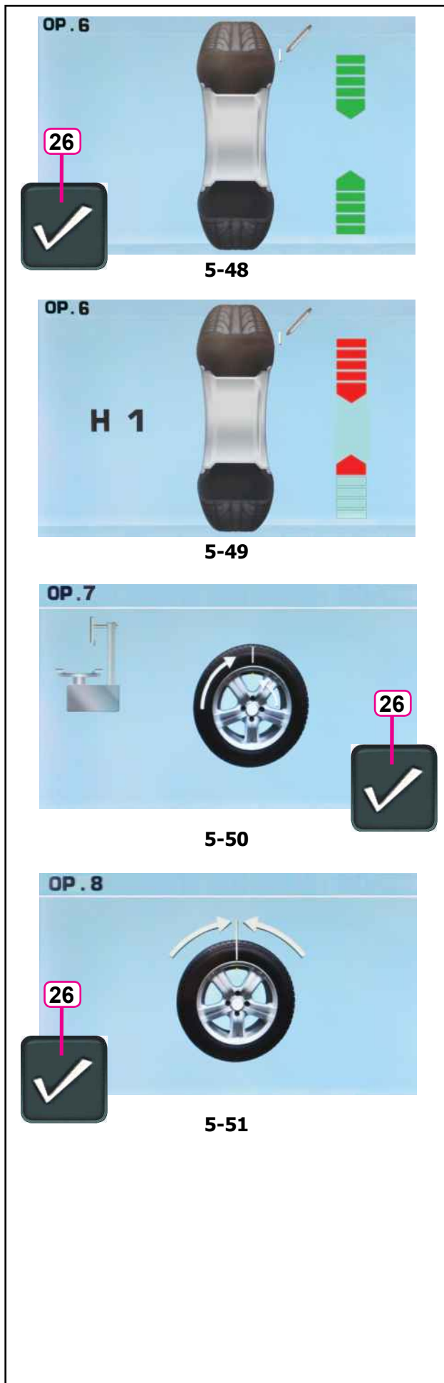
Figure 5-48 OPTIMISATION “OP.6” (second measuring run with tyre)
