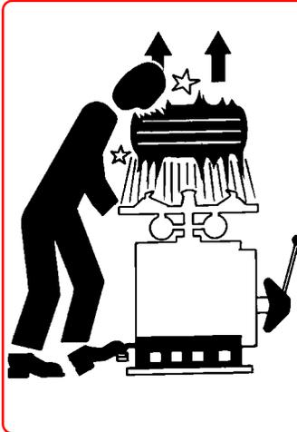
An exploding tire and rim may be propelled upward and outward with enough force to cause serious injury or death. This tire changer is not a safety device and will not restrain exploding tires and rims.
