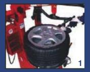
Pneumatic Bead Assist (PBA) device lets a single operator safely and effectively meet the challenges of changing low profile tires, run flats and other performance tires with extremely stiff sidewalls. The PBA actually consists of a power pneumatic cyllinder that drives three separate mechanisms: top bead roller, bead depressor and bottom bead roller. Here's how PBA works:
