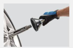
Electromechanical Power Clamp clamps wheels quickly and easily, reducing force applied by operators for increased accuracy and performance.
