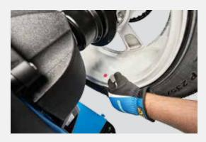
Accurate positioning of adhesive weights avoids misplacement to accelerate every job.
