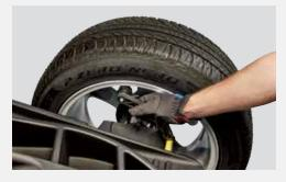
**2D SAPE Data Entry** The 2D SAPE gauge arm enables semi-automatic input of rim diameter and offset.
