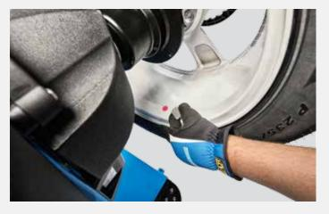
**easyWeight** Pinpoint red laser provides fast, accurate, easy positioning of adhesive weights on the wheel, identifying exact weight placement locations for increased accuracy and productivity.
