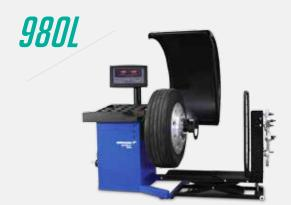
The geodyna<sup>®</sup> 980L heavy-duty wheel balancing system is designed to handle the balancing needs of trucks, buses, RV's, and Light Truck/Automobile tires. The geodyna<sup>®</sup> 980L is equipped to handle from the smallest of wheels, 12" (30.5 cm) to heavy-duty 25" (63.5) and "super-singles".
