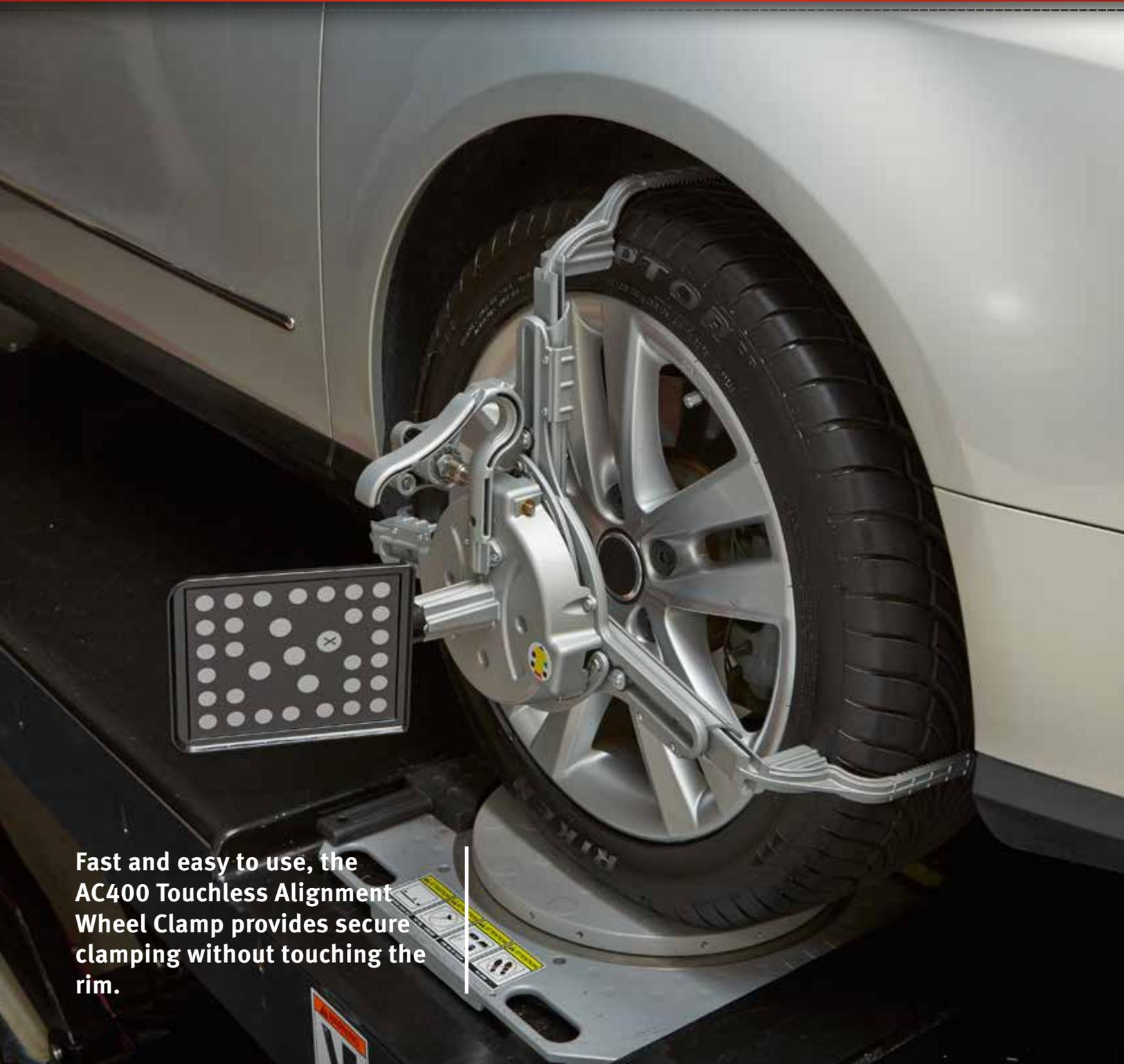
Fast and easy to use, the AC400 Touchless Alignment Wheel Clamp provides secure clamping without touching the rim.
