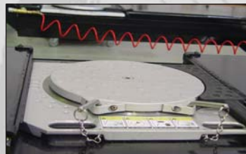
Optional stainless steel turnplates slide on a UHMW layer preventing deck scratching.
