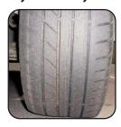
Camber or Toe Wear: Indicates misalignment due to loose, worn or bent steering linkage components. Many camber & toe wear problems can be traced to spring fatigue, which causes the vehicle's frame to ride closer to the road. Once the vehicle is
