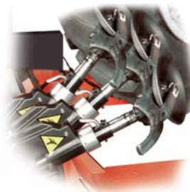
The tool support can be adjusted to three positions
