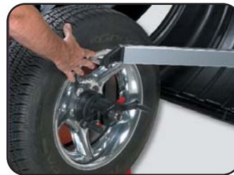
Outer Auto-Assist Data Input Arm Measures Wheel Width. (VPI System III only)
