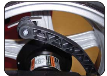
Inner Auto-Assist Data Input Arm also places tape weights behind spokes or on inner edge of wheel.
