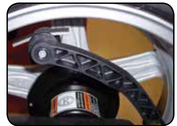
Inner Auto-Assist Data Input Arm also places tape weights behind spokes or on inner edge of wheel
