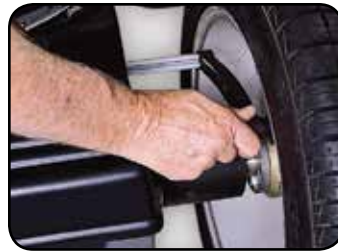
Inner Auto-Assist Data Input Arm Measures Wheel Distance and Diameter
