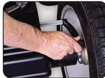
Inner Auto-Assist Data Input Arm Measures Wheel Distance.
