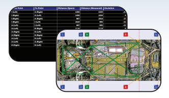
**Point to Point Measuring** Point to Point measuring with color coded results provides damage interpretation.
