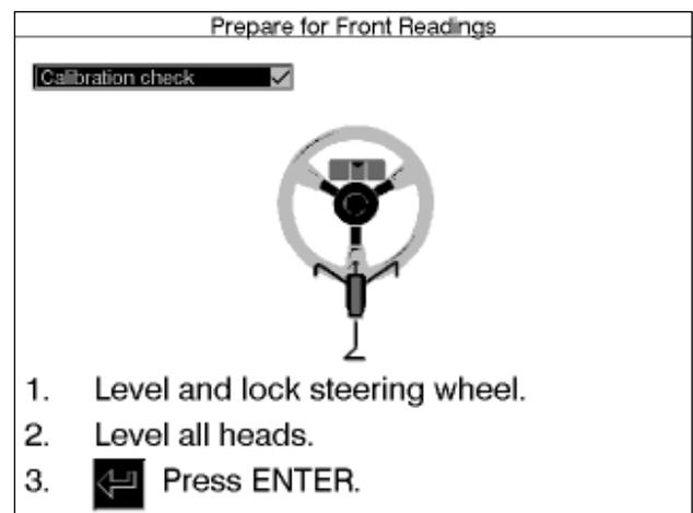
Figure 12 -- Calibration Check is Performed
