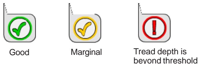
Figure 18c - Tread Depth Indicators
