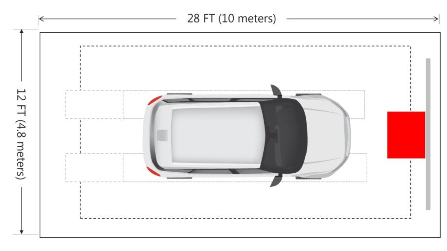
Wheel alignment bay length and width requirements are less than the ADAS bay size requirements. In addition, some systems calibration require the vehicle to be on the GROUND not 10" of the ground or on an alignment rack. <u>View the Honda Lane Watch System Calibration</u>
