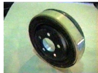
Figure 13 Dampen vibrations during the Machining operation. Excessive tightness of silencer on drums may result in minor chatter.
