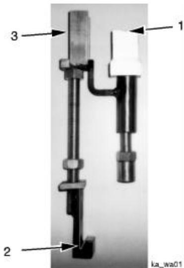
Pick-up attachment for the calibration arm
