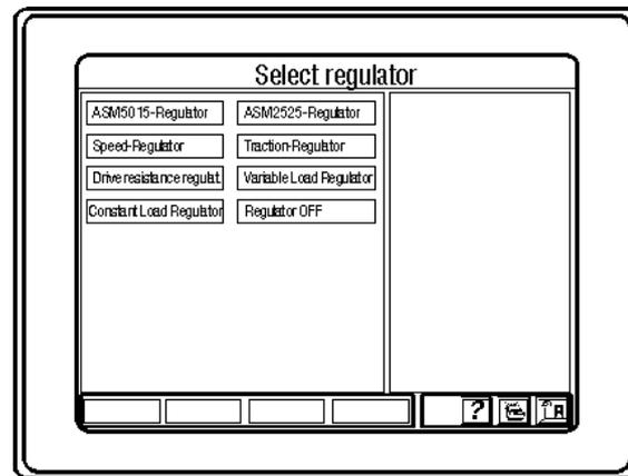
The following regulators are most important for the operation of the ASM
