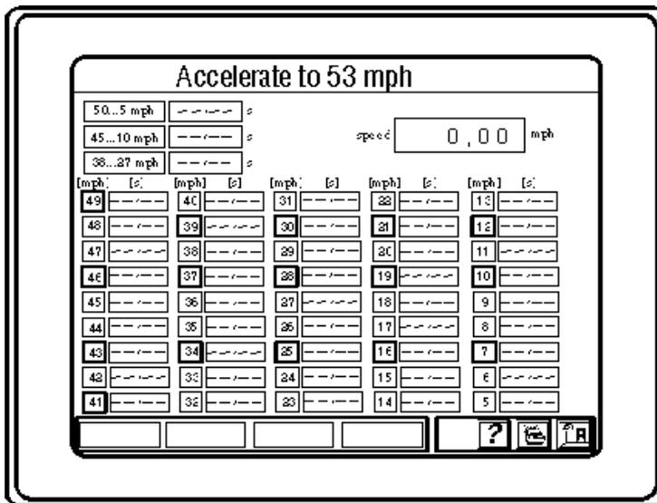
The test stand is accelerated with an external drive to ca. 53 mph. After the drive has been switched off the roller set is allowed to coast down. The Variable-Load-Regulator is triggered at 50 mph as shown in Figure 6-1. The times in the respective speed windows is determined by decelerating the test stand.
