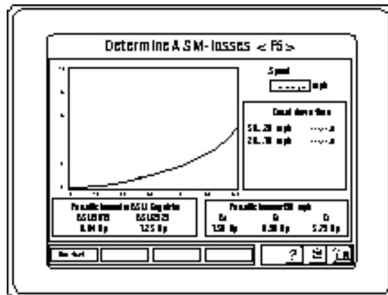
The ASM-losses are also determined by a coast down trial. The rollers are accelerated to a speed somewhat higher than 30 mph through the built in motors. After the speed has been reached the regulator will be switched off. An internal stop watch monitors the time it takes to reach the speed of 20 mph. This trial will also be conducted for the speed range 20 mph - 10 mph.
