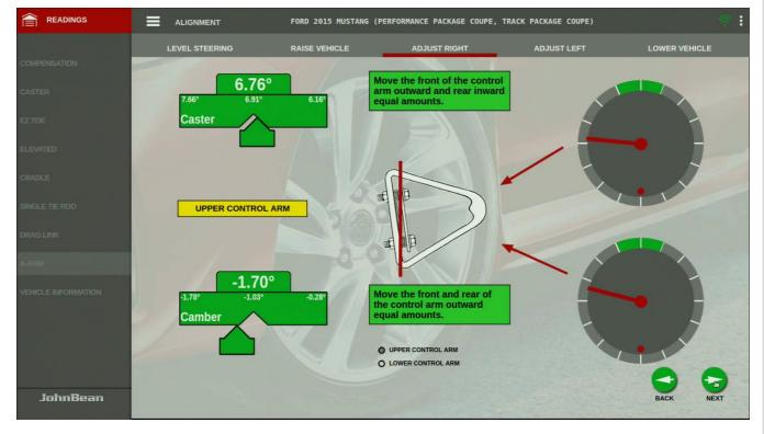
Upper and or lower control arm shim, slots, or eccentric cam bolts.
