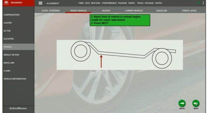
Taking the load of the suspension makes the adjustment easier and faster
