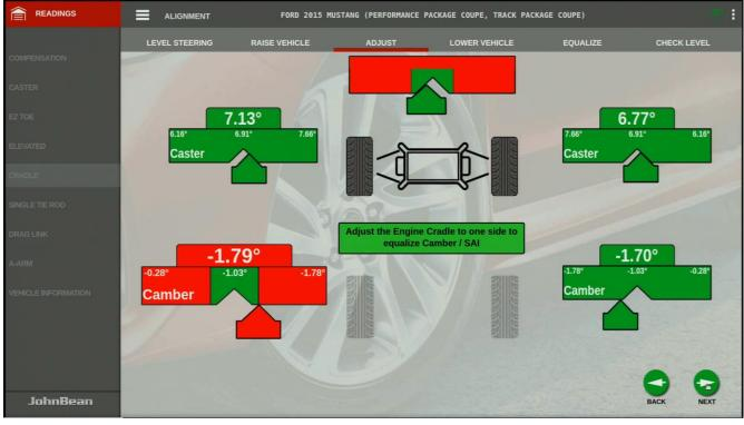
Cradle adjustment is normally required after a transaxle replacement or repair, post front end collision work, or after hitting a curb
