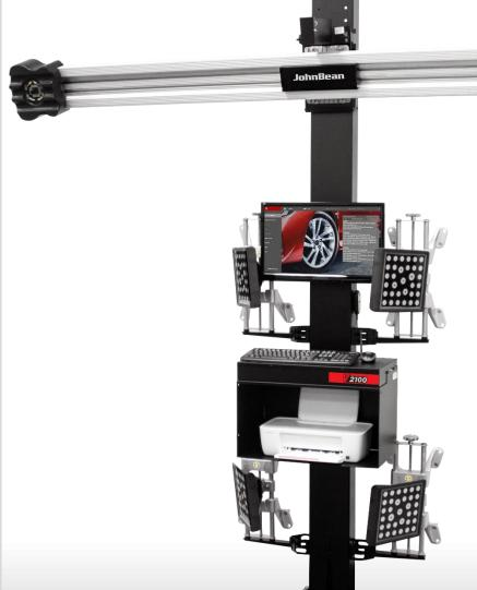
Utilizing advanced imaging technology, the John Bean® V2100 provides accurate, realtime measurements - reducing setup and measurement times while generating serious productivity benefits. Matched with our latest software, the V2100 wheel aligner will have your technicians getting readings in a matter of minutes.
