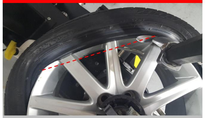
Incorrect procedure, the tire is not in the drop center, excessive pressure is applied to the mount\demount head, PROSpeed<sup>™</sup> stops the machine
