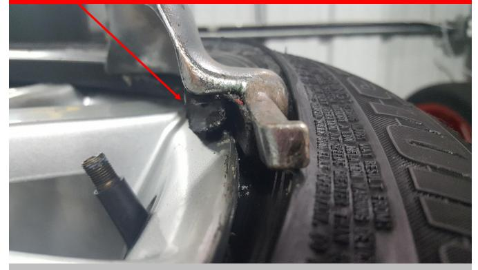
This is a run flat tire, on a standard single or two speed table top tire changer. The tire and wheel assembly exceeds the machines capability.
