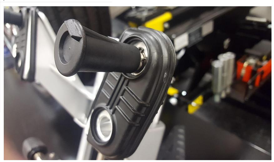
The plastic wheel protectors rests against the rim's edge to position the clamp on the wheel.
