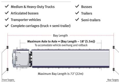
Bay length is the separation of the reference targets installed on the floor. Without limitations, the maximum allowed bay length is 72 feet and therefore the maximum length vehicle that can be measured is one with 54 feet between the first and last axle. Typically the size of the customer space determines the bay length. In that case, the maximum axle to axle length is the 18 feet less than the distance between the reference targets.
