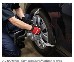
without touching the rim; clutch-limited clamping force ensures secure and consistent attachment.
