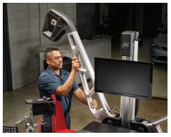
Folding camera beams provide a lower center of gravity for improved stability while protecting cameras during transport.
