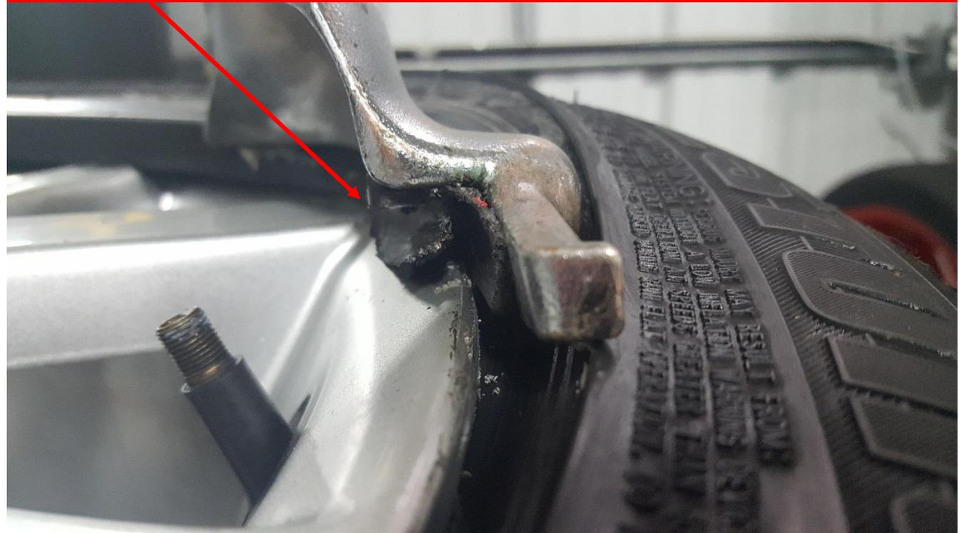
This is a run flat tire, on a standard single or two speed table top tire changer. The tire and wheel assembly exceeds the machines capability.
