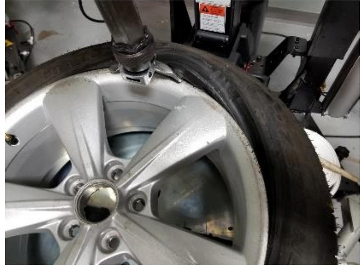
Once traction point is approximately at the 4 o'clock position notice that tire changer speeds up and load decreases. The motor sound will increase in pitch as speed increases.
