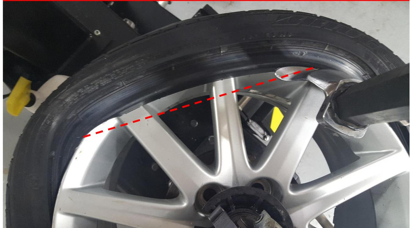
Incorrect procedure, the tire is not in the drop center, excessive pressure is applied to the mount/demount head, PROSpeed™ stops the machine
