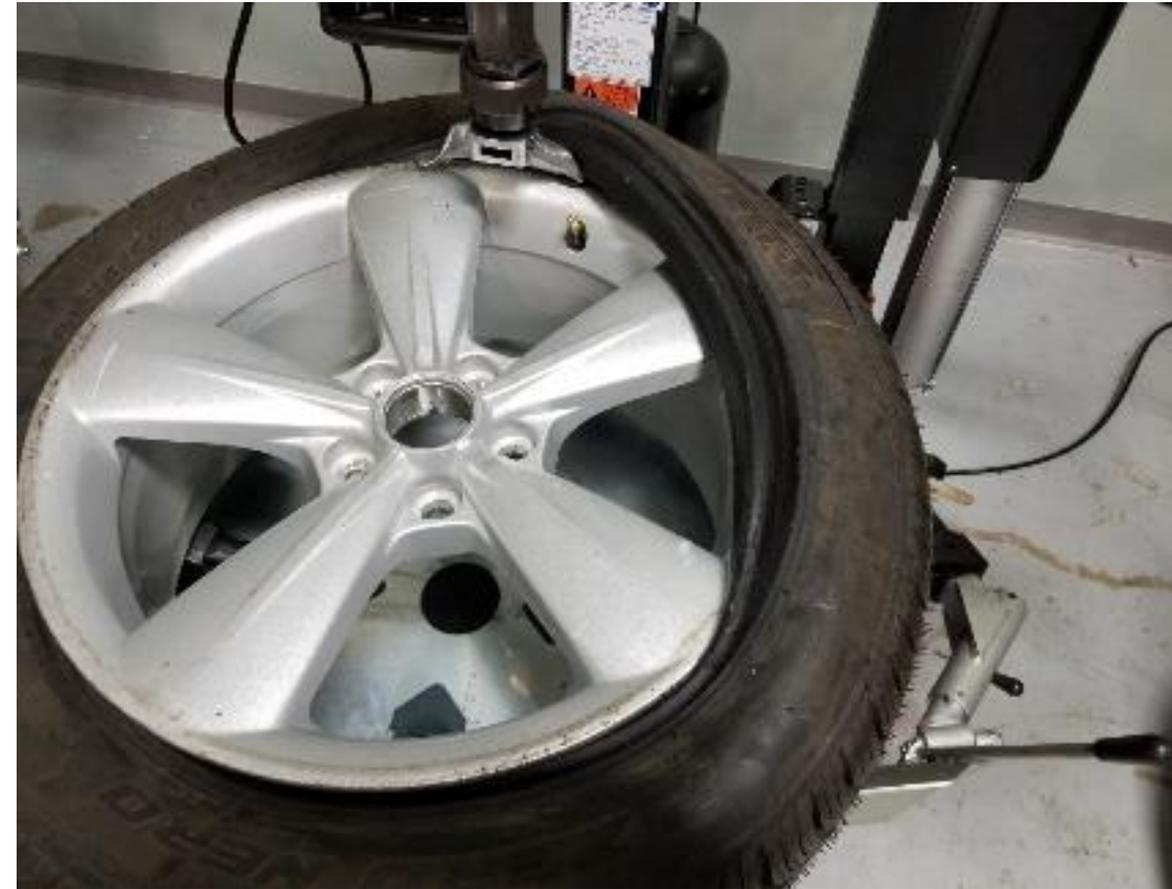
Use mount/demount head to begin mount procedure, do not slam bottom bead on. Motor will run at its fastest speed during this operation.
