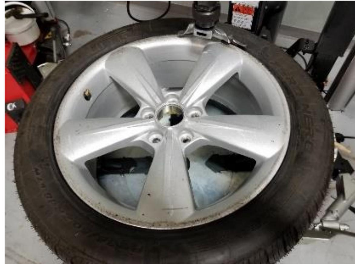
After pull over, remove tire bar, begin to rotate, and notice tire changer initial slow speed.
