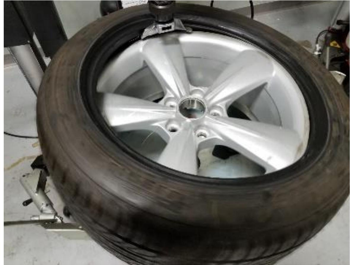
Begin mounting the top bead, deliberately force bead out of drop center. Tire changer will slow down as load increases.
