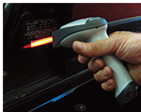
Optional VIN Code Reader scans and automatically inputs the VIN into the aligner, saving time and eliminating the possibility of operator error.
