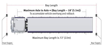
Bay length is the separation of the reference targets installed on the floor. Without limitations, the maximum allowed bay length is 72 feet and therefore the maximum length vehicle that can be measured is one with 54 feet between the first and last axle. Typically the size of the customer space determines the bay length. In that case, the maximum axle to axle length is the 18 feet less than the distance between the reference targets.
